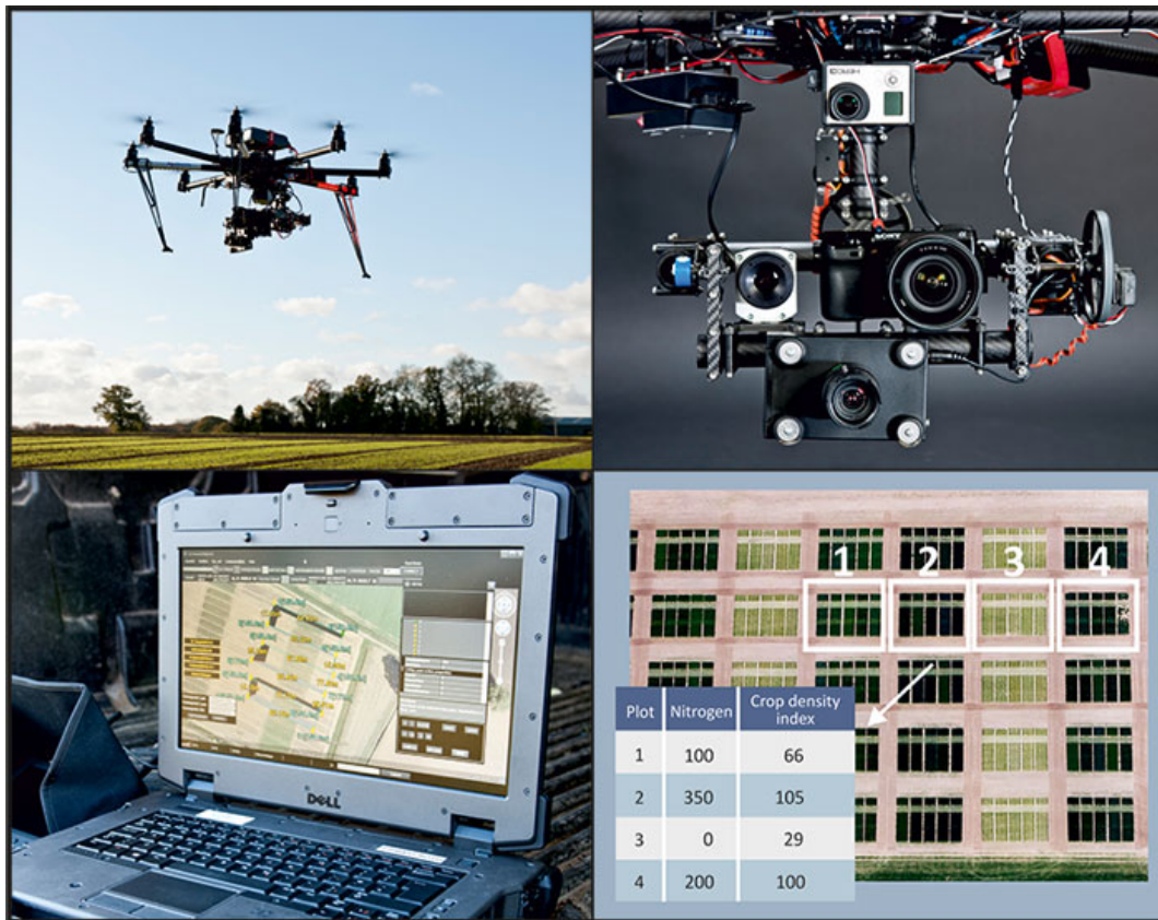
Figure 6: The unmanned aerial vehicle (UAV) to be used on a weekly basis during the 2013-2014 field season to monitor canopy status (NDVI) and stress (thermal imaging) for all varieties/N-treatments in the diversity trial
